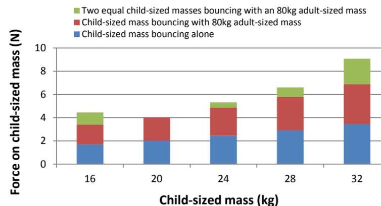
Figure 2. Comparison of maximum forces exerted on child-sized mass during one, two and three person bouncing
