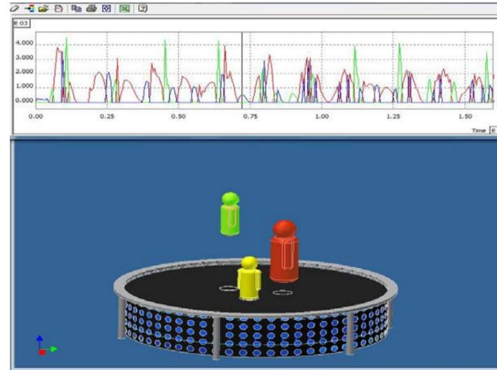
Figure 1. Autodesk Inventor biomechanical model. The line colour in the graph corresponds with the colour of the mass (except for the blue line which represents the yellow mass).
